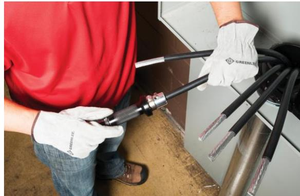
The GTS-1930 Saber is developed with a one-way barring handle that allows users to maintain control of the cutback throughout the stripping process, ensuring the blade does not come into contact with the conductor. There are no additional tools needed for cut back set up. The tension grip depth stop has a four-inch laser-etched stop for precise articulation of cable cut back.
